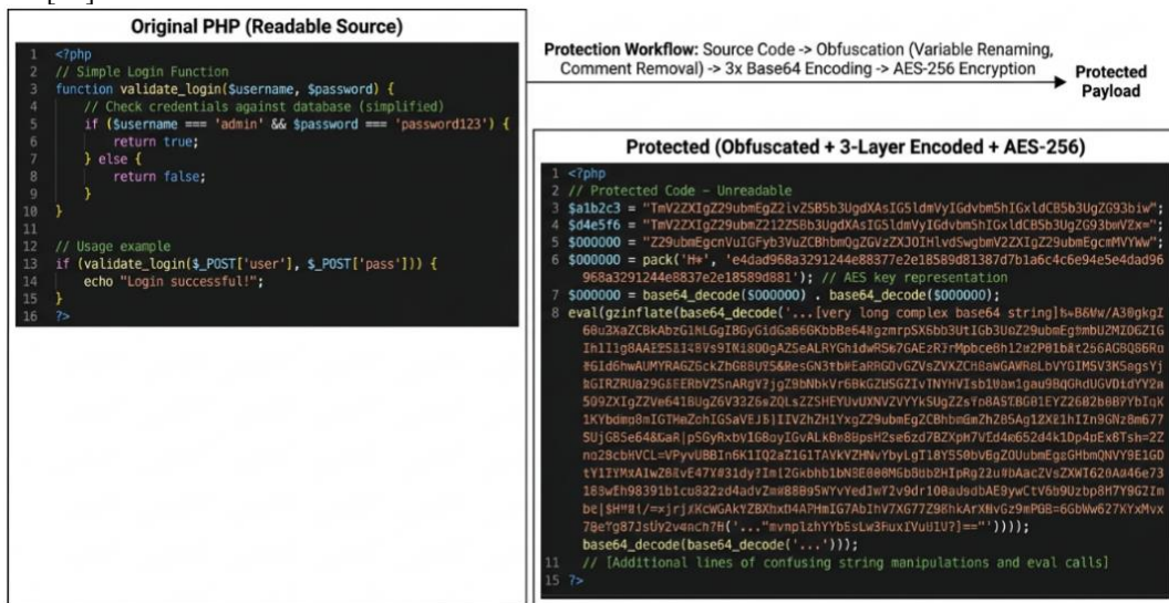
Figure 2. Sample PHP code transformation through a multi-layer protection pipeline.
